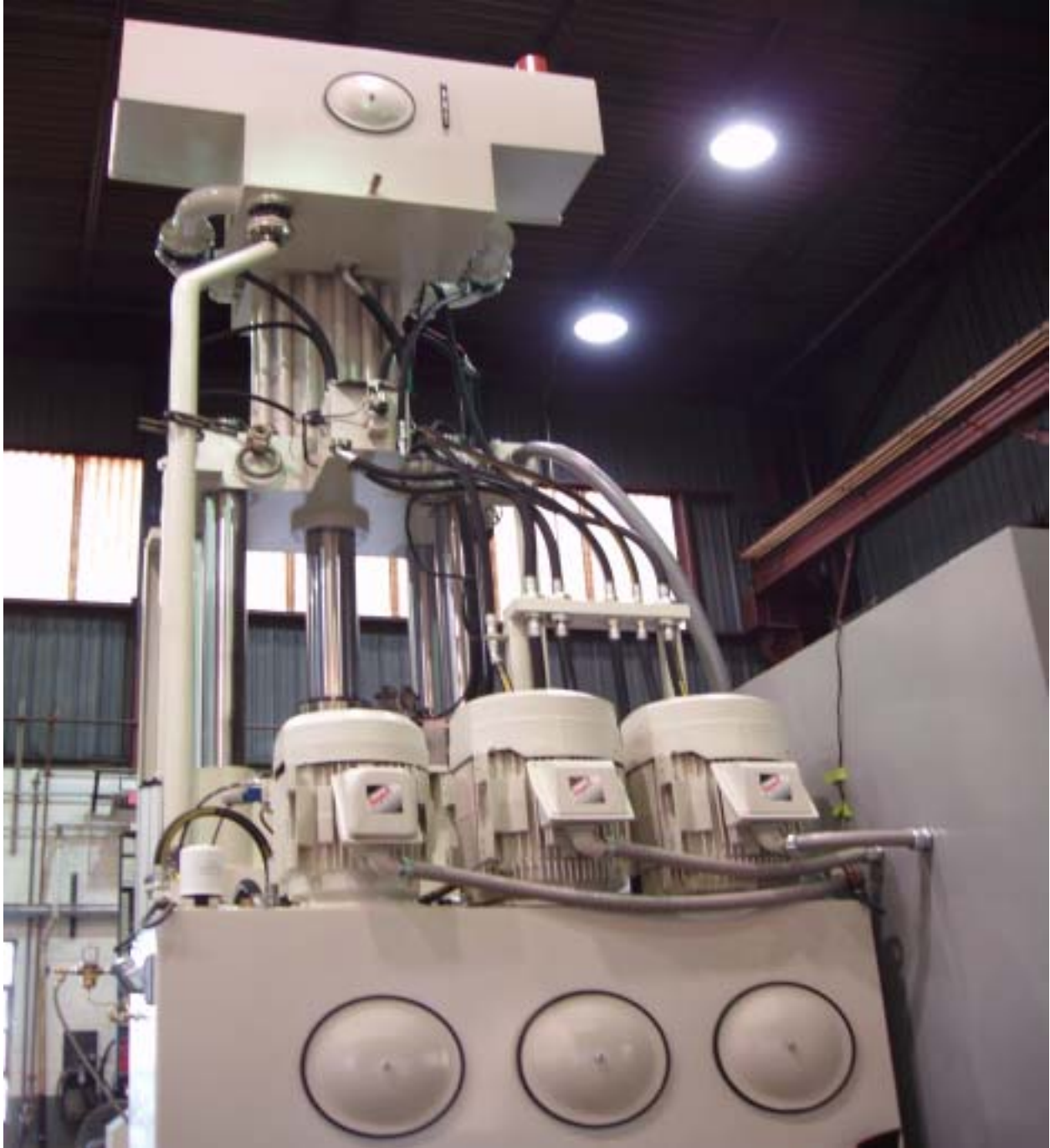
View from the rear of the press showing the Three Motor/Pump Groups. Power Unit capacity was 415 gallons.
