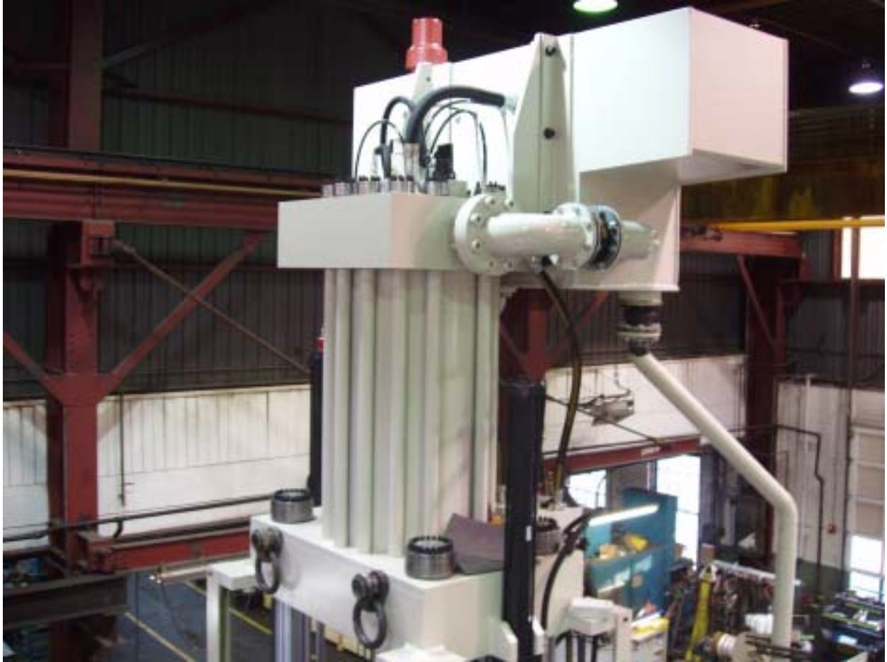
Main Cylinder designed and built by Greenerd Press & Machine Co., Inc. Photo also shows Prefill tank mounted off Top Cap of the Cylinder for providing oil flow during Rapid Down Stroke. Prefill valve with flexible coupling shown on side of Main Cylinder.
